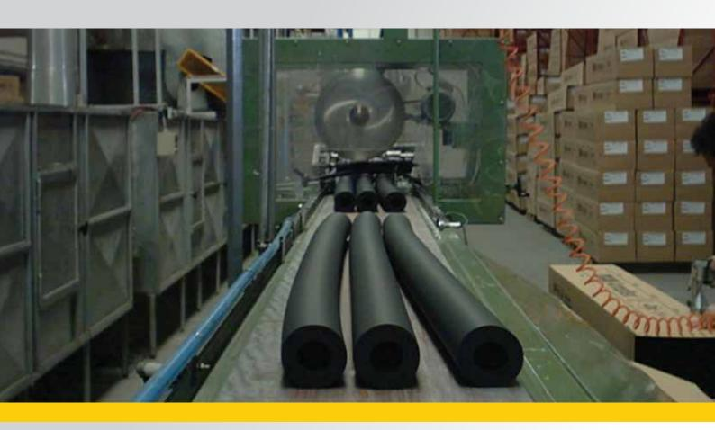
Elastomeric Rubber is elastomeric rubber based thermal insulation material that has closed porosity and even cell structure. It can be manufactured in the forms of sheet and pipe in different size and with different technical properties and varied facing materials according to the intented use and the place of use. It is used for thermal insulation and condensation control.
